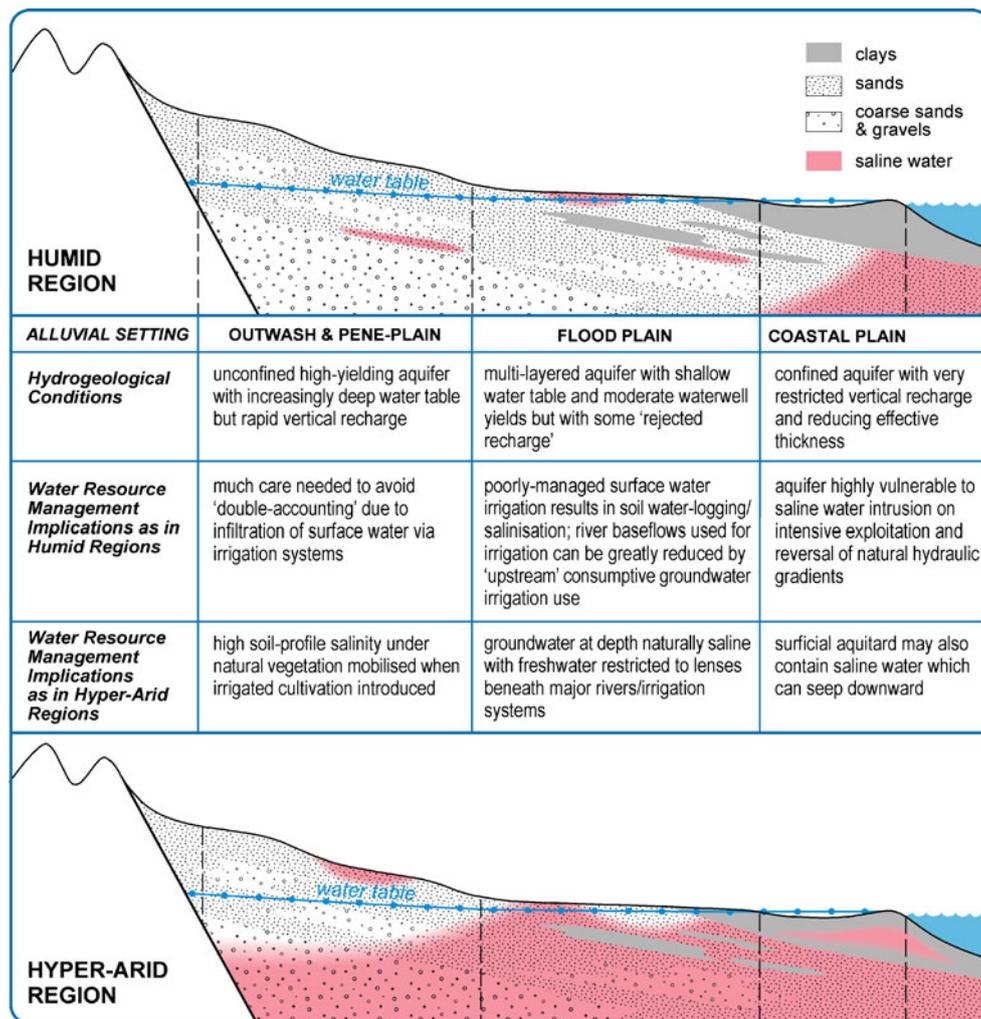
**Fig. 1** Schematic long-profile of a typical alluvial groundwater system in a humid region detailing the variation in groundwater-surface water connectivity and salinisation hazards
