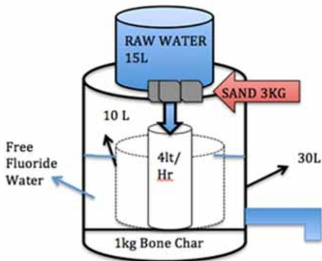
The household bone char filter is made of two blue plastic baskets. The raw water basket is of 15 L capacity. Filtered through a layer of bone sand (3 kg), the water drips into the second tank. This process takes about 30 minutes. The users can keep the process going if they keep refilling the first tank with raw water.
