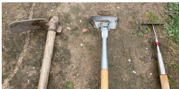
From left to right: an eye-hoe and two scuffle hoes (stirrup hoe in the middle and collinear hoe to the right)
