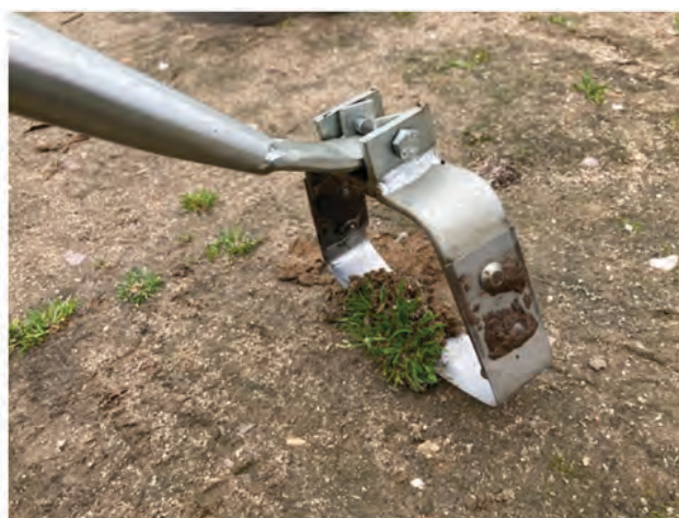
Stirrup hoe forth cutting motion (left) and back cutting motion (right). Notice the hinge that permits the cutting blade angle to change
